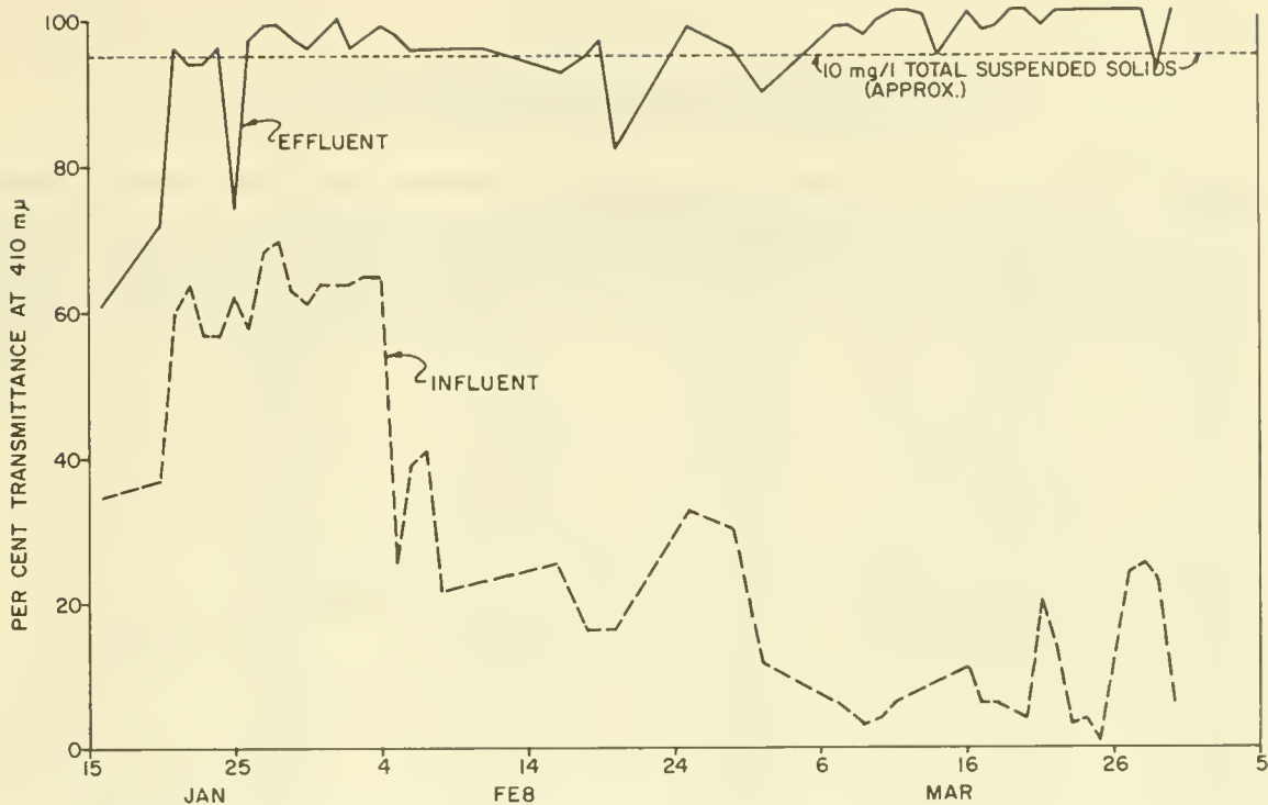
FIGURE 51-PER CENT TRANSMISSIONS OF WATER BOY INFLUENT AND EFFLUENT SAMPLES DURING FIRST THREE MONTHS OF 1970
